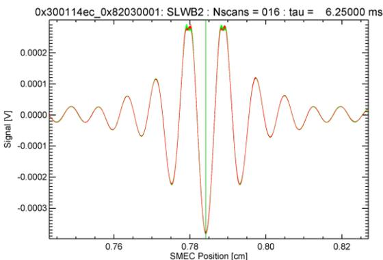
Figure 4.1: Interferograms clipped off the position of ZPD.
