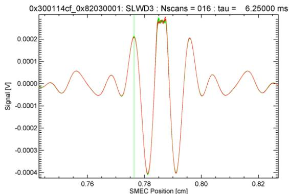
Figure 4.2: Interferograms clipped at the position of ZPD.
