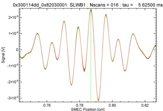
Figure 4.3: Well-compensated interferograms; SLW Array.
