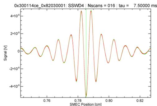
**Figure 4.6: Interferogram orientation when the Telescope port is dominant; SSW Array.**
