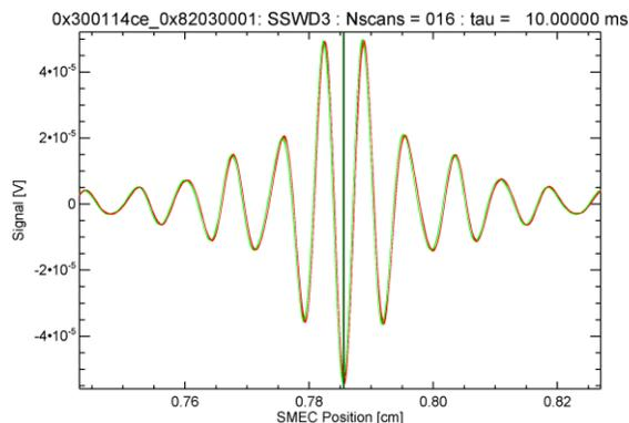
Figure 3.2: Interferograms generated after the first iteration of the binary search.
