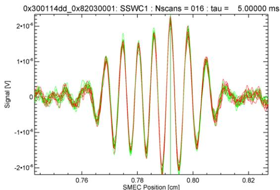
Figure 4.4: Well-compensated interferograms; SSW Array.
