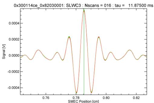
**Figure 4.5: Interferogram orientation when the Telescope port is dominant; SLW Array.**
