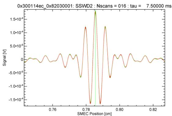
**Figure 4.8: Interferogram orientation when the SCAL port is dominant; SSW Array.**
