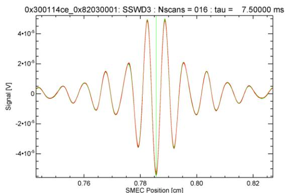
Figure 3.4: Interferograms generated after the third iteration of the binary search.
