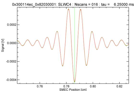
**Figure 4.7: Interferogram orientation when the SCAL port is dominant; SLW Array.**
