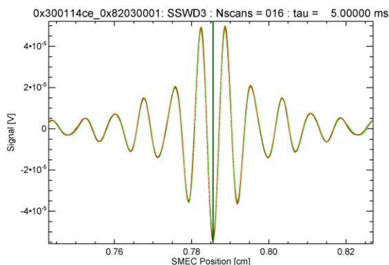
Figure 3.3: Interferograms generated after the second iteration of the binary search.
