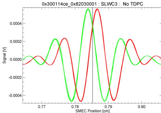
**Figure 2.1: Interferograms recorded for channel SLWC3.** No attempt has been made to compensate for the delay induced by the readout electronics and the bolometer thermal response. Note the separation between the forward scans (green) and the reverse scans (red).
