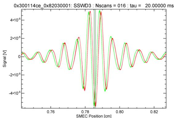
Figure 3.1: Interferograms generated after the initial guess of the thermal time constant. The median forward ZPD and median reverse ZPD are shown as vertical black lines.
