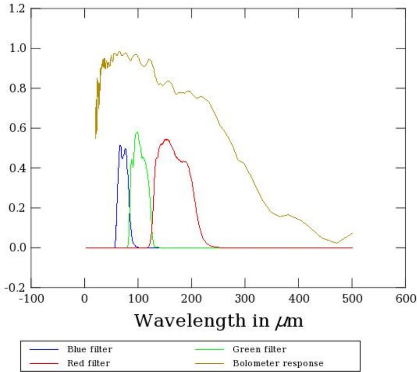
**Figure 3-1:** Filter transmissions and bolometers response
