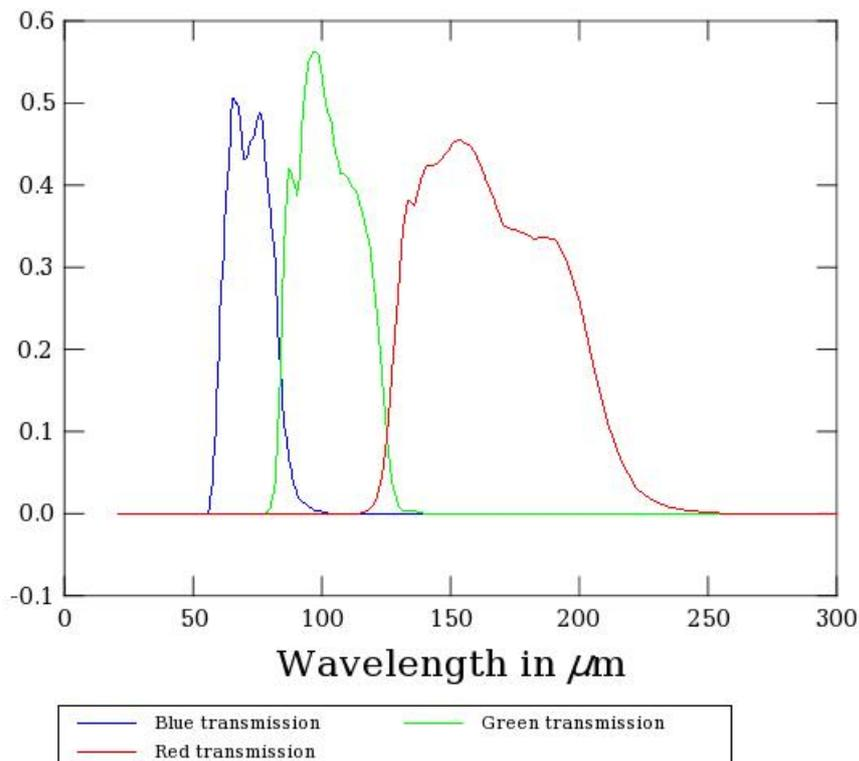
**Figure 3-2:** Optical transmissions for the three bands of PACS
