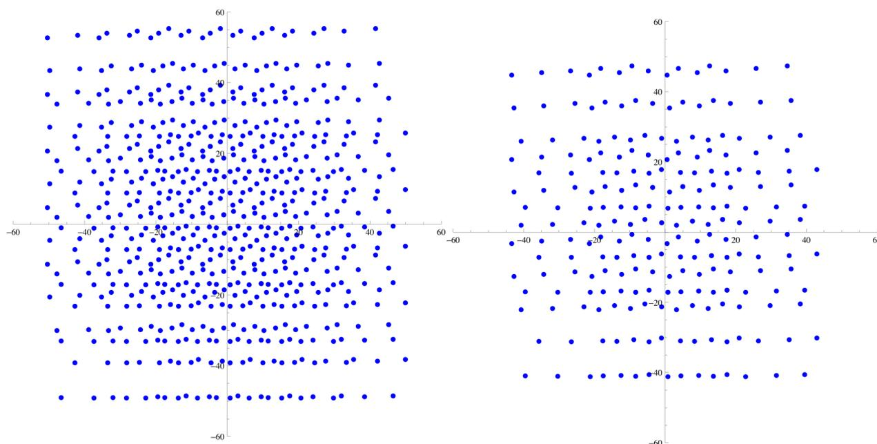
Figure 8: Spatial sampling by all PACS spaxels when using a 5x5 raster with step size 14.5''/16'' for the blue (left) and a 3x3 raster with step size 22''/24'' for the red (right)
