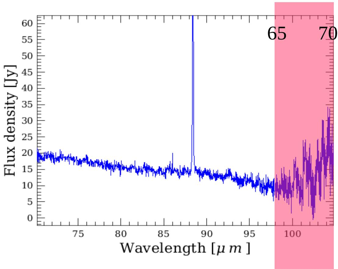
Figure 10: Spectral leakage in band B2B: beyond 98 $\mu m$  the response is very low, and spectral features from order 3 (65-70 $\mu m$ ) are superimposed on the spectrum
