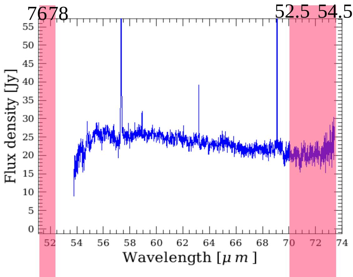
Figure 11: Spectral leakage in band B3A: beyond 70 $\mu$ m, the order 4 (52,5-54.5 $\mu$ m) spectrum is added to the 70-73 $\mu$ m order 3 spectrum. The 51-52 order 3 spectrum also shows the 76-78 $\mu$ m order 2 spectrum.
