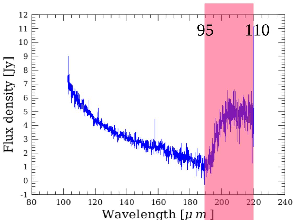
Figure 9: Spectral leakage in band R1: the spectrum between 190-220μm has an unreliable (line) flux calibration, and shows superimposed spectral features from order 2 (95-110μm).
