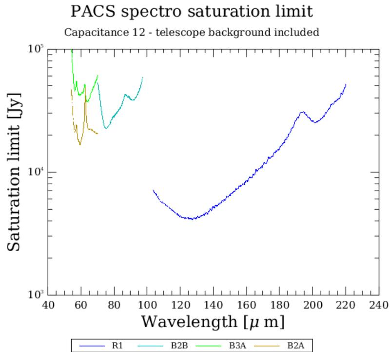
Figure 6: Saturation limit for the largest integrating capacitance.
