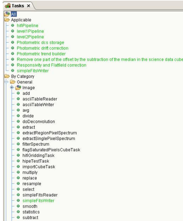
Figure 32. Tasks available for a given DP session variable are automatically made available in the "Tasks" view. Applicable tasks are shown in the Applicable Tasks folder.
