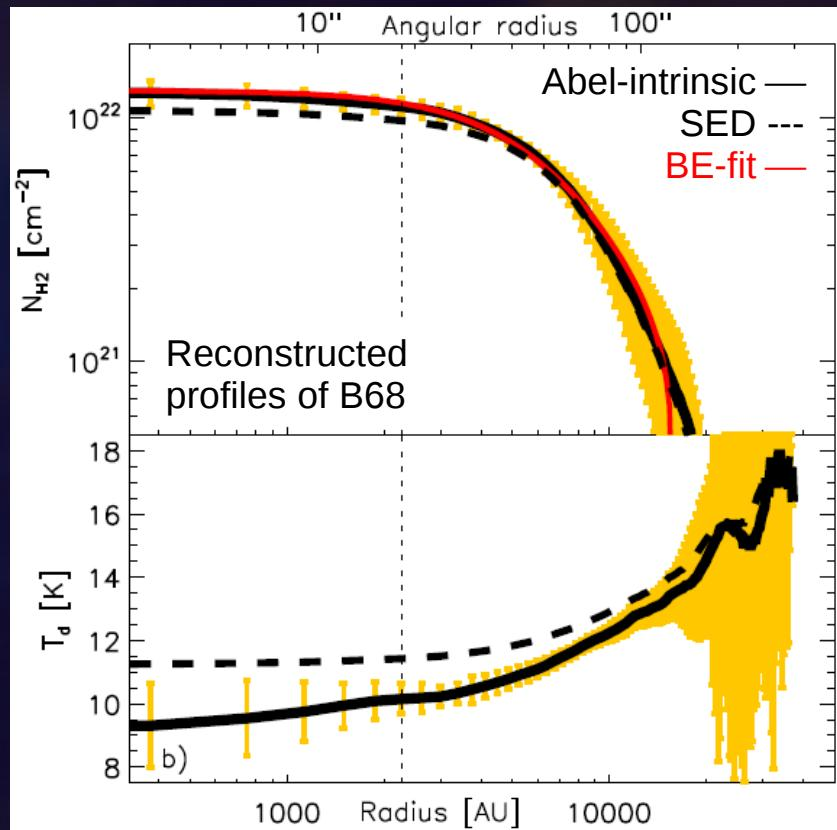
$N_{\text{H}_2}$  and  $T_{\text{d}}$  profile reconstruction based on Abel transformation technique (Roy et al., subm.)
