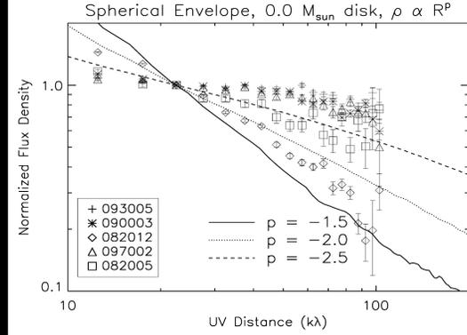
**Figure 4:** PBRs visibility amplitudes compared to spherical envelope density profiles. Without an additional compact source the PBRs with flat visibilities are most consistent with  $p = -2.5$ .
