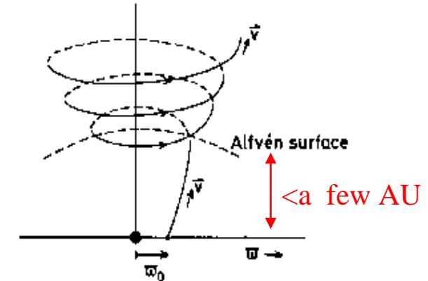
Figure 1.3: Development of the azimuthal field. With each rotation of the field line a loop of field is added to the flow at the Alfvén surface.
