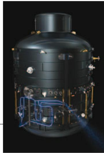
The cryostat vacuum vessel containing the superfluid helium tank. The gas is ejected into space. The cryostat vacuum vessel is cooled down to about 70K ( $-203^{\circ}\text{C}$ ) by radiating heat into space.
