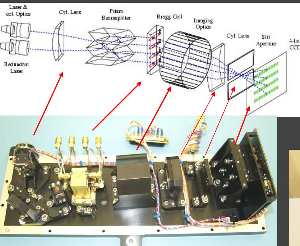
Source module   Bragg-cell   Imaging optics   Cyl. lens   CCD
