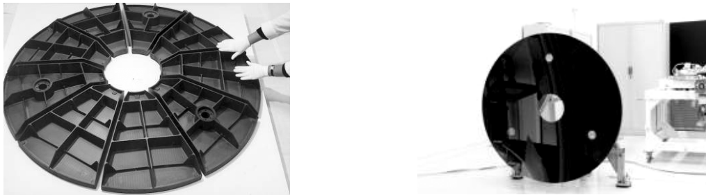
Figure N°14: \Phi 1.35\text{ m} HERSCHEL demonstrator (before brazing and after, brazing, machining and polishing)
