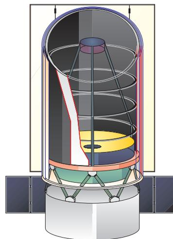
Figure 1. Conceptual design of the SPICA mission with a 3.5 m primary mirror cooled to 4.5 K.
