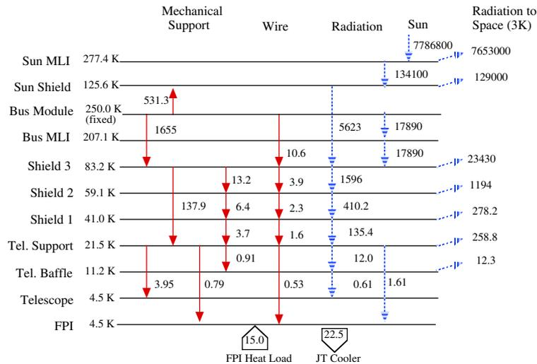
Figure 3. Heat flow (unit: mW) diagram of the SPICA mission cooled by radiation and mechanical coolers. Filled arrows show the heat flow by conduction and dotted arrows show the heat flow by radiation. We assume a structure of the conceptual design (Figure 1)
