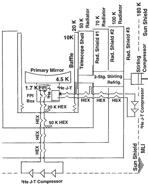
Figure 2. Schematic diagram of the cryogenic system of SPICA. The telescope is enshrouded with multi-layered radiators. One set of a JT cooler (with <sup>4</sup>He) and a two-stage Stirling cycle is used to cool both the telescope and focal plane instruments to 4.5 K. Another set of a JT cooler (with <sup>3</sup>He) and a two-stage Stirling cycle is used to cool far-infrared detectors to 1.7 K.
