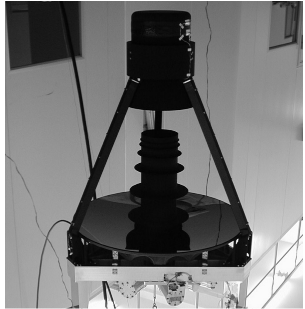
Figure 4. The telescope assembly of ASTRO-F. Both the primary and secondary mirrors are made of SiC.
