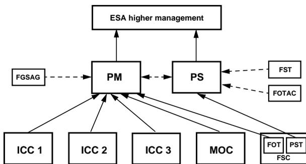
Figure 5. A box diagram of the FIRST ground segment during the development phase. For the ICCs, which are PI responsibility, there are formal links through agreements between the PIs and ESA. The FST is the FIRST Science Team, PM the Project Manager, PS the Project Scientist, PST the PS Team, and FOT the FSC Operations Team.
