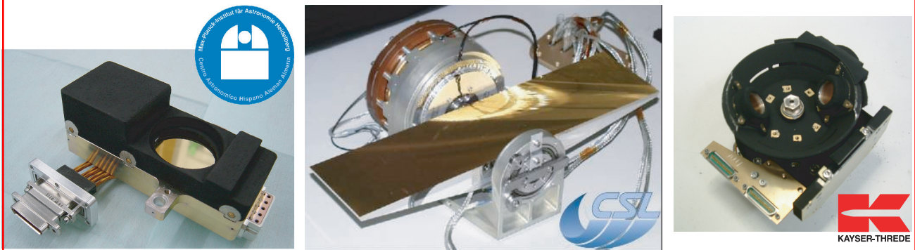
Figure 5. PACS cryomechanisms. Left: Qualification Model of the focal plane chopper. 13, 14 The chopper is used for sky modulation and also to deflect the detector field of view toward 2 internal calibration sources. Center: Qualification Model of the grating unit. A torquer motor is used to actuate the grating angle which is measured with sub-arcsecond precision by an Inductosyn angular resolver. Right: Qualification Model of one of the two filter wheels. The motor is the same design as the grating torquer.
