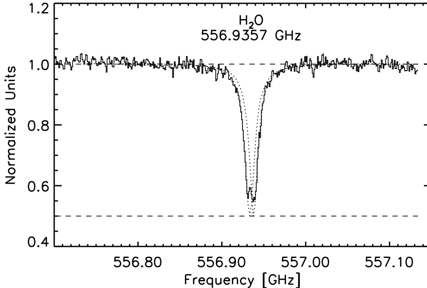
Remark: The water could not be removed completely from the sample cell for the reference measurements causing an absorption in the line center!
