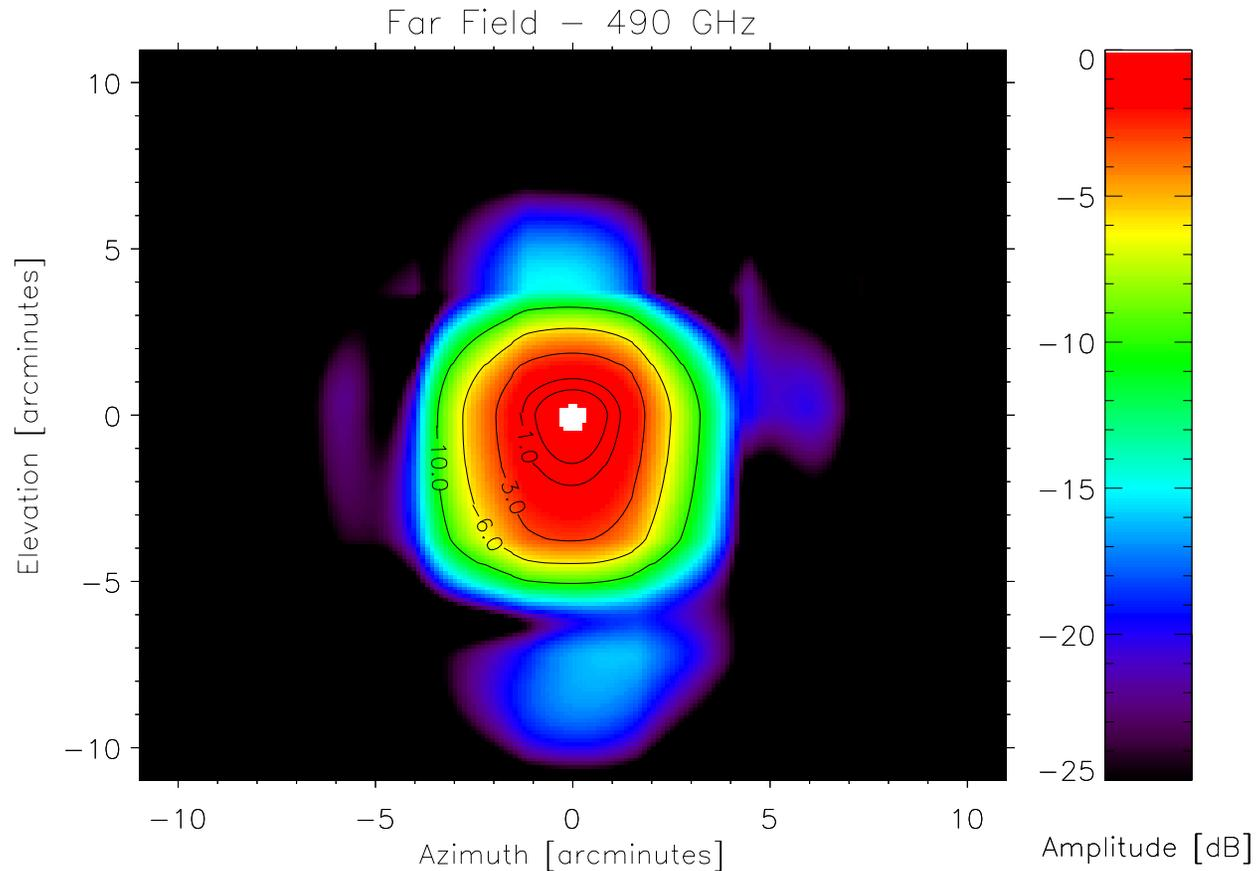
Verification of Co-alignment of SWAS beams to be within a few arcseconds
