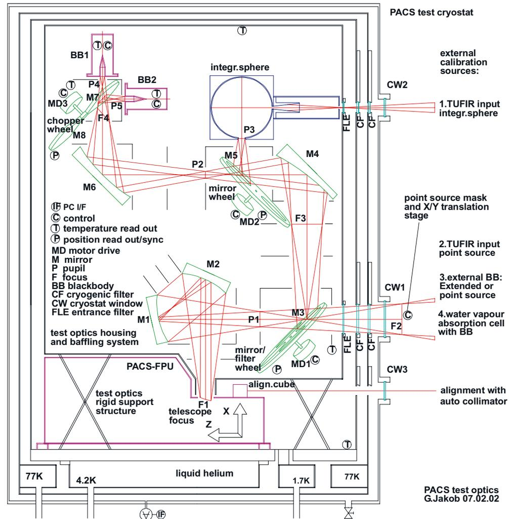
**Fig. 10 PACS test optics and Herschel telescope simulator schematic**
