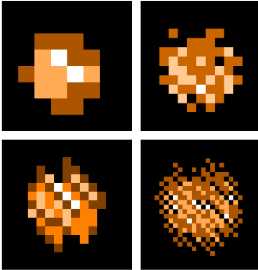
Figure 3.20: Intermediate (top) and Full (bottom) spatial sampling coverage maps for SLW (left) and SSW (right) from a real SPIRE FTS mapping observation. The sky spectral pixel (spaxel) sizes are 35 arcsec (top left), 17.5 arcsec (bottom left), 19 arcsec (top right), 9.5 arcsec (bottom right). The number of bolometer hits in each sky pixel are encoded with colour. The holes in the maps, due to dead bolometers, depend on the spacecraft attitude (the focal plane position angle), the grid centre, the pixel scale.
