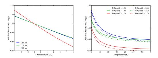
Figure 5.8: The variation of effective beam area relative to the beam area used in the pipeline ( $\alpha_{pip} = -1$ ). The areas are plotted against source spectral index (left) and against grey body temperature for two values of the grey body index  $\beta$  (right). See Table 5.5 and 5.6.
