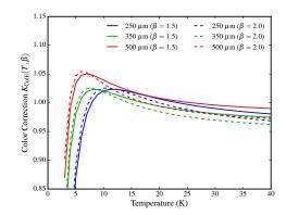
Figure 5.5: Colour correction parameters for point sources ( $K_{\text{ColP}}$ , left) and extended sources ( $K_{\text{ColE}}$ , right), vs. assumed modified blackbody source temperature. The colour correction factors are plotted for two values of emissivity index,  $\beta = 1.5$  and  $\beta = 2$ .
