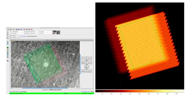
Figure 3.15: Parallel Mode footprint image example as displayed in HSpot (left). NGC 7293 is imaged in "Nominal" scan direction with a coverage area of  $54' \times 72'$ . A comparison between observer's requested area and real instrument coverages, normalised to 1, is shown on the right, the green rectangle is the original observer requested area. SPIRE coverage is the darker area on the left.
