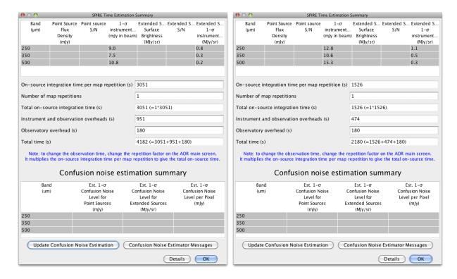
Figure 3.6: Large Map time estimation and sensitivity for a filed of  $60' \times 60'$  and one repetition for a cross-linked (scan A and B, left) and single scan direction (right).
