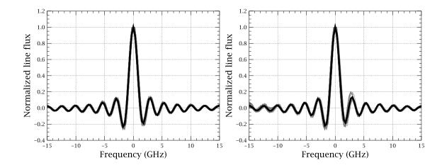
Figure 3.25: The FTS instrumental line shape, the *sinc* function. The average line shape (in black) for the two central detectors from unresolved CO lines in the HR spectrum of NGC 7027, SSWD4 (left) and SLWC3 (right). The grey curves show the line shapes for all 30 observations of NGC 7027.
