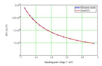
Figure 5.2: Typical plot of f(V) vs. V (for a nominal 350  $\mu$ m bolometer). The blue points correspond to the bolometer model and the red line is the fitted function using Eq. (5.6).
