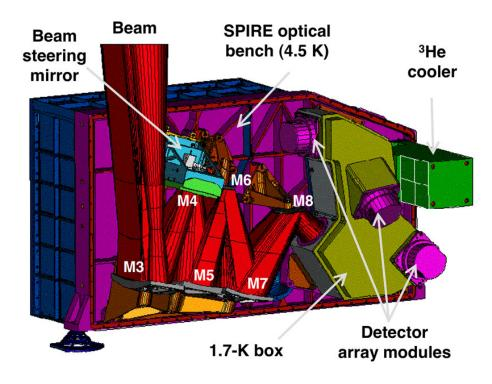
Figure 2.3: SPIRE FPU: photometer side layout.
