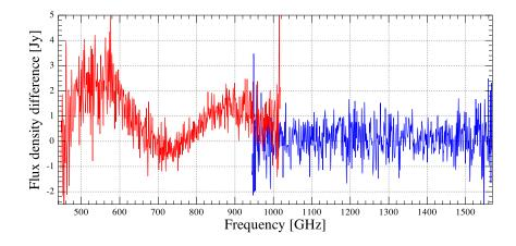
Figure 6.4: The difference between the HR and LR point-source calibrated spectra for the centre detectors of the H+LR observation 1342253971. SSW is essentially flat, whereas there is a bumpy distortion in the difference for SLW. The peaks seen at 500 and 900 GHz are introduced by artefacts in the LR data. The LR data were interpolated onto the HR frequency scale before subtraction from the HR data.
