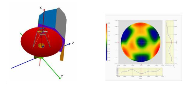
Figure 5.9: View of the model geometry (left) and reconstructed telescope pupil optical path difference map from environmental ground measurements by *Herschel* Observatory industrial contractors (right).
