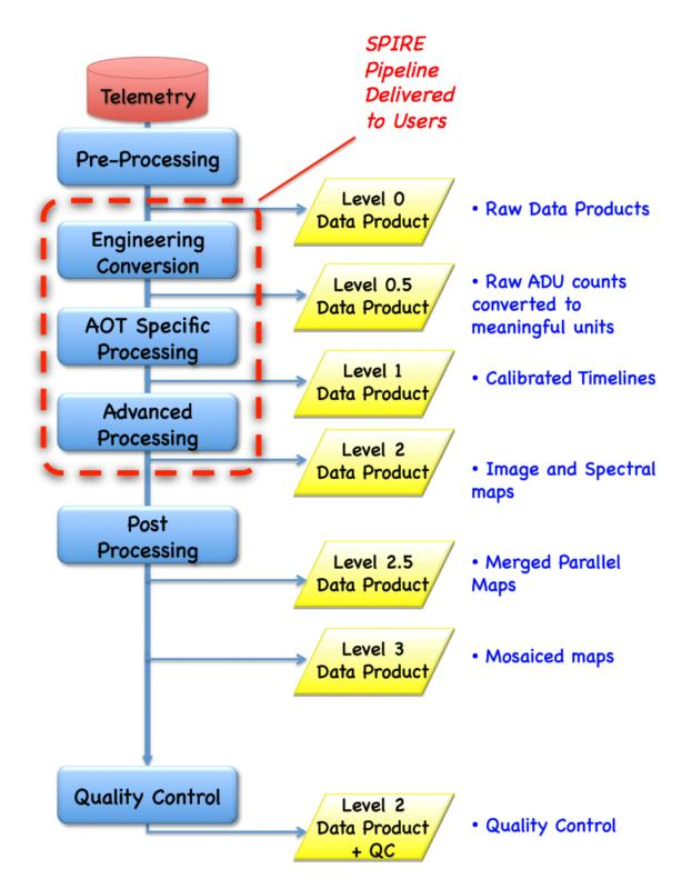
Figure 8.2: The processing levels of the SPIRE pipeline and user deliverables. Level 2.5 and Level 3 are only available for the Photometer and for subsets of observations.
