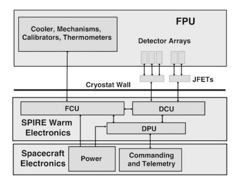
Figure 2.1: SPIRE instrument architecture
