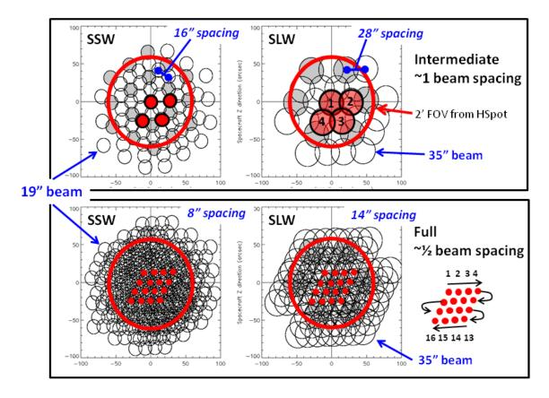
Figure 3.22: The FTS mapping pattern with intermediate image sampling for SSW and SLW (4-point jiggle, top) and full sampling (16 point jiggle, bottom). The red circle shows the 2' diameter unvignetted field of view of the FTS. The spacing of the beams is indicated for each of the detector arrays and the two image sampling modes. The red dots show the central detector of each array at the 4 jiggle positions (top) and the 16 jiggle positions (bottom).
