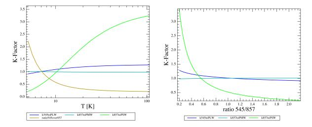
Figure 5.12: Left: the three colour correction factors  $K_{\rm HFI \to SPIRE}$  and the ratio  $R_{\rm HFI}$  as a function of dust temperature, assuming a fixed dust emissivity index  $\beta=1.8$ . Right: the three colour correction factor  $K_{\rm HFI \to SPIRE}$  as a function of the ratio  $R_{\rm HFI}$ , for  $\beta=1.8$ .
