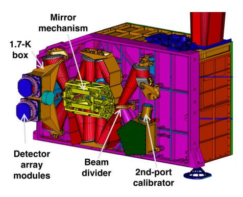
Figure 2.5: SPIRE FPU: spectrometer side layout.
