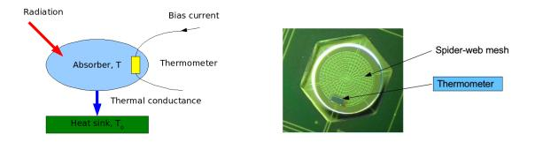
Figure 2.7: Basic principles of bolometer operation (left) and a magnified view of a SPIRE bolometer (right). The thermometer size is  $10x100x300 \mu m$ .
