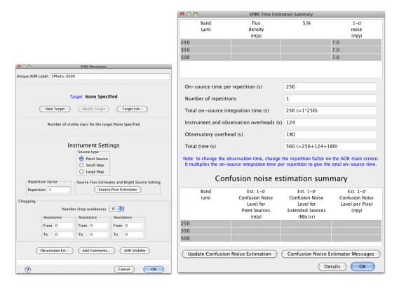
Figure 3.10: HSpot user inputs for Point Source mode (left) and the HSpot time estimation for Point Source mode (right).
