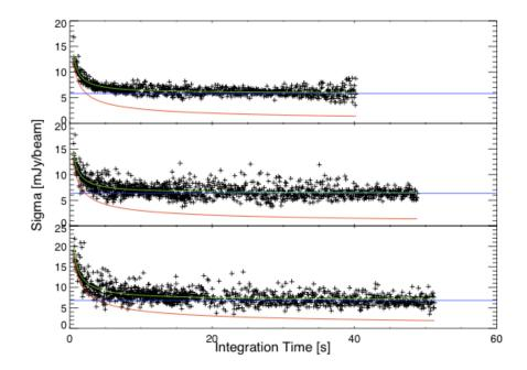
Figure 3.24: Pixel noise vs. integration time for all pixels in deep SPIRE photometer fields. The derived instrument noise is shown in red, the confusion floor is show in blue and the total noise is in green. Taken from Nguyen et al. (2010).
