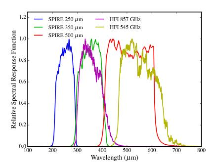
Figure 5.11: Relative Spectral Response Functions,  $R(\nu)$ , for the five wavebands: *Planck*HFI 545 GHz & 857 GHz, and *Herschel*SPIRE 250  $\mu$ m, 350  $\mu$ m & 500  $\mu$ m bands.
