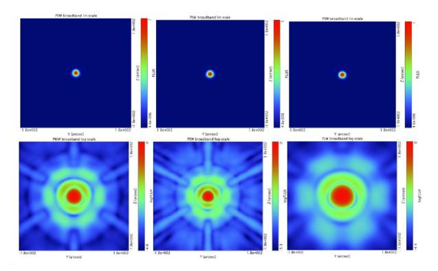
Figure 5.10: Theoretical photometer beams for 250, 350, and 500  $\mu$ m (left, centre, and right, respectively), with linear scaling (top row) and logarithmic scaling (bottom row).
