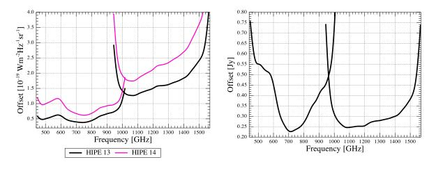
Figure 7.1: Additive continuum offsets for extended-source (left) and point-source calibration (right). The extended calibration offsets were significantly underestimated for processing before HIPE v14 due to the missing far field feedhorn efficiency correction (see Section 6.1 for more details).
