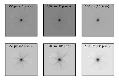
Figure 5.6: Log scale images for the empirical SPIRE beam at 250, 350, and 500  $\mu$ m from left to right respectively. The top row uses a 1" pixel scale for all maps, and the bottom row uses the nominal SPIRE map pixel scales of 6, 10, and 14" from left to right respectively. The beam maps extend out to 750" radius.
