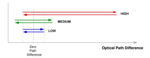
Figure 3.18: Diagram to show how the SMEC moves (in terms of optical path difference) during one repetition for High, Medium and Low spectral resolution. The low resolution SMEC scan range is always covered during High or Medium resolution observations.
