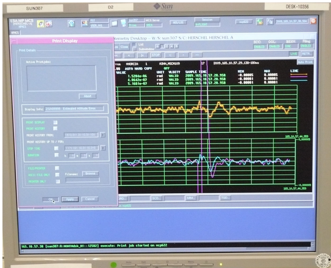
Figure 1.4. The telemetry received at MOC showing the oscillation in gyro response as the cryocover swung open.
