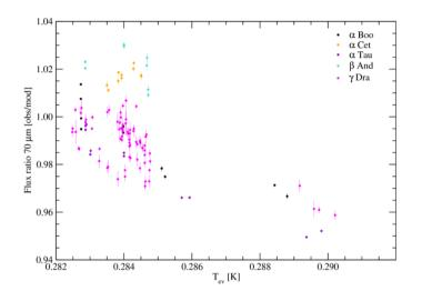
Sensitivity seen to vary with PACS evaporator temperature. Also effects of changing mirror temperature and emissivity seen! Can be removed (see LHS) for stellar calibrators.
