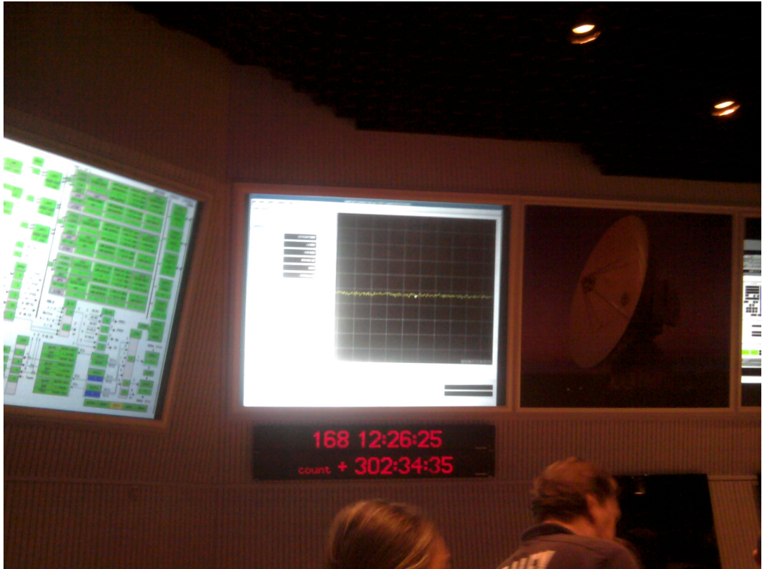
Figure 1.23. The screen in the Main Control Room at MOC showing the output from the frequency analyser. This would normally show a strong signal at the frequency of the Herschel transponder. The flat line shows that the signal from the Herschel transponder had dropped to zero after switch-off. The point at which the transponder signal dropped to zero marked the end of the Herschel mission.
