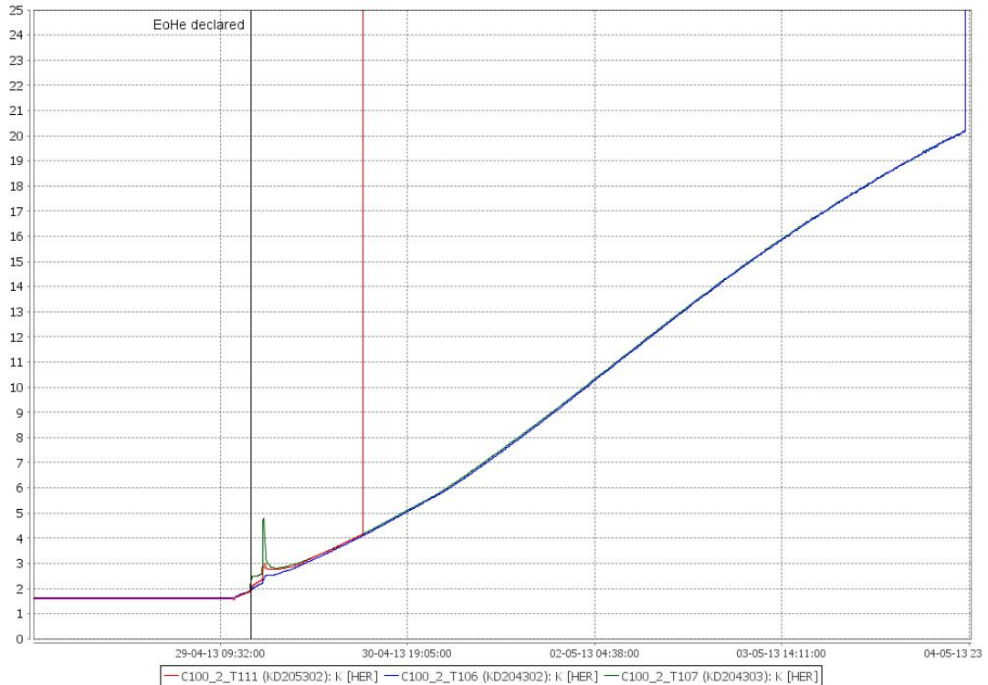
Figure 1.18. Cryostat temperatures from April 28th to May 4th 2013. The graph is initially stable at 1.7K before starting to rise around 12:30UT on April 29th, marking the evaporation of the last drop of helium. The solid black line marks the point at which an internal temperature of 2.0K was reached, marking the formal criterion for declaring End of Helium. The plot shows the slow rise of the cryostat temperature after End of Helium (EoH) was declared. Temperature curves are shown for the T111 (red curve), T106 (navy blue curve) and T107 (green curve) sensors, which were in different positions inside the cryostat. As each sensor went out of limits it shoots vertically off the scale. Approximately five days after boil-off the temperature reached 20K and the T106 and T107 sensors went out of limits simultaneously (Graphic courtesy: MOC).
