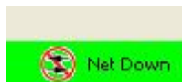
Figure 5.2. The net-down symbol means HSpot cannot access the HSC servers. You may still enter target and AOT information when the net is down but you cannot calculate observing time estimates, obtain visibility windows, obtain background estimates, and may not be able to download images or catalogues.
