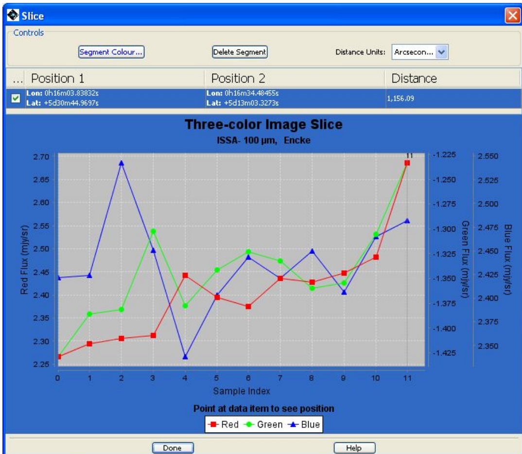
Figure 20.22. The graphic of the background across a slice of the image. In this case a three-colour image has been used, so three colours and lines are plotted.
