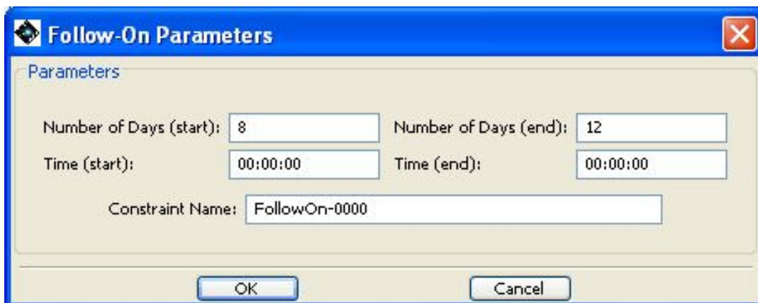
Figure 16.23. The window to define the Follow-On parameters for Follow-On observations. In this case the window for execution is defined to be between 8 and 12 days after the previous AOR has ended.
