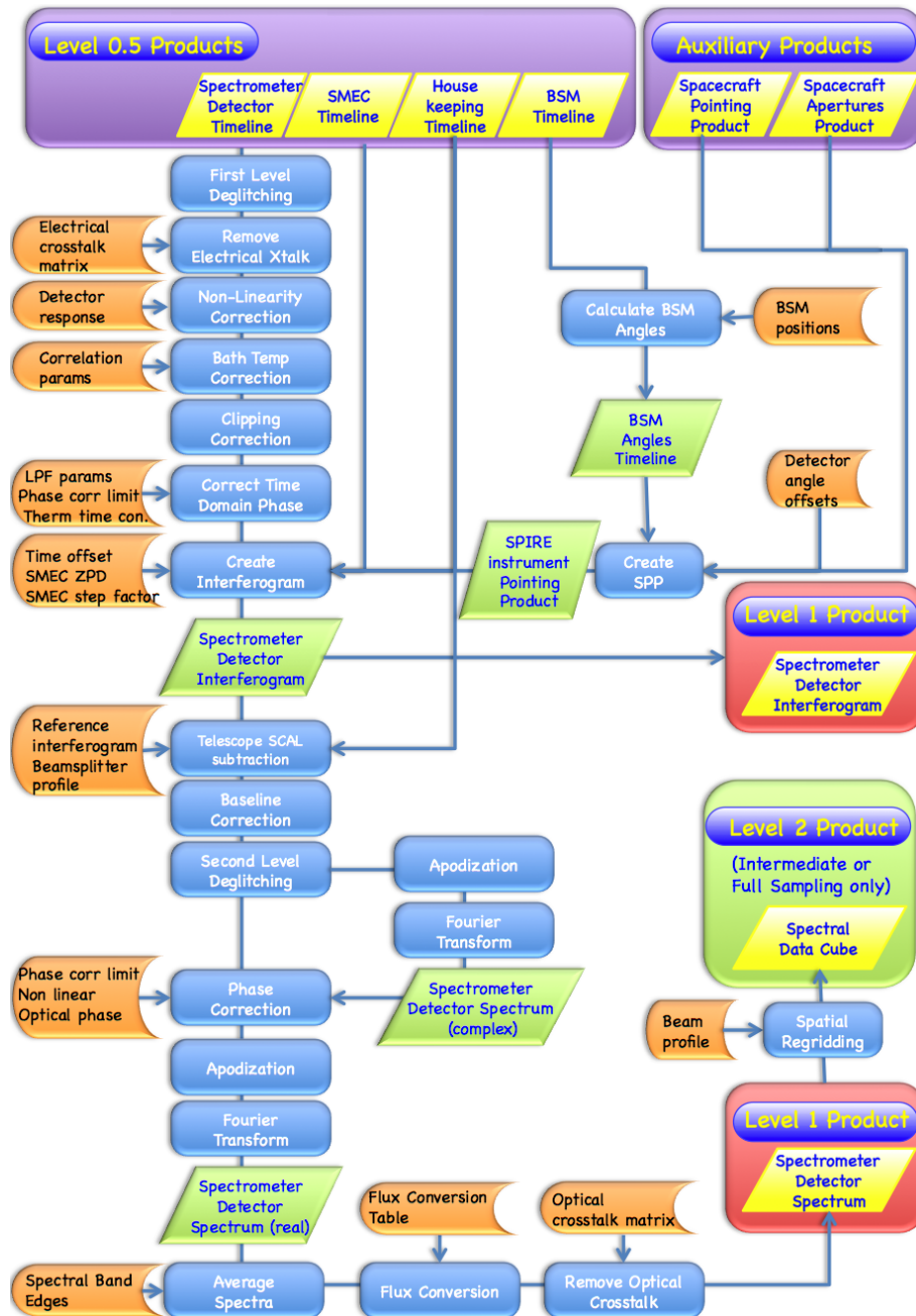
Figure 3.13. The SPIRE Spectrometer pipeline.
