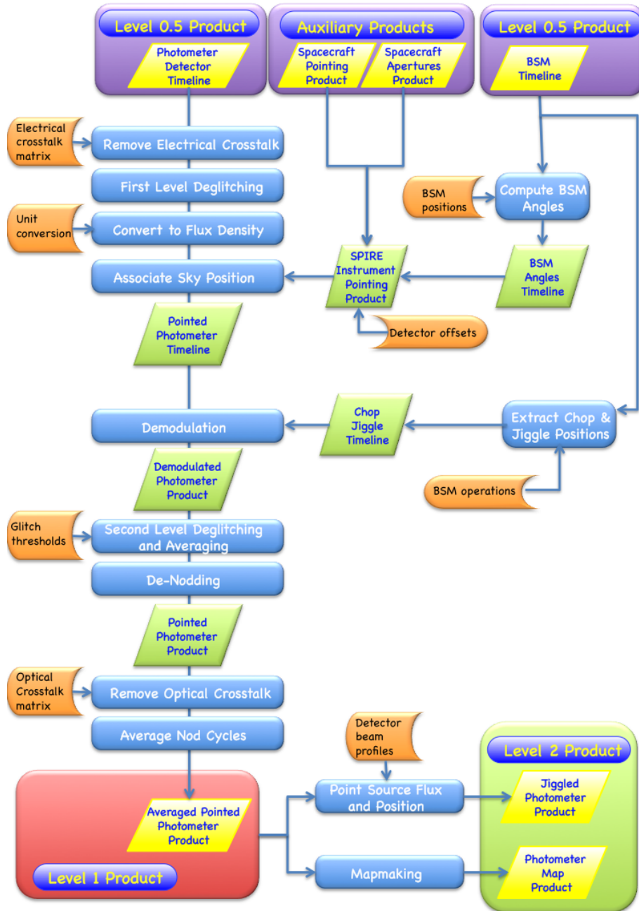
Figure 3.1. The SPIRE Jiggle mode pipeline.
