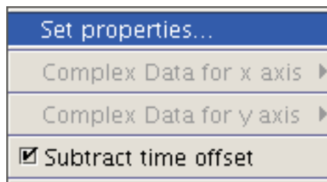
Figure 4.9. Preferences: This drop-down menu gives access to the zoom- and pan-properties, the display rules for complex data, and the control over time offset subtraction on the X-axis.
