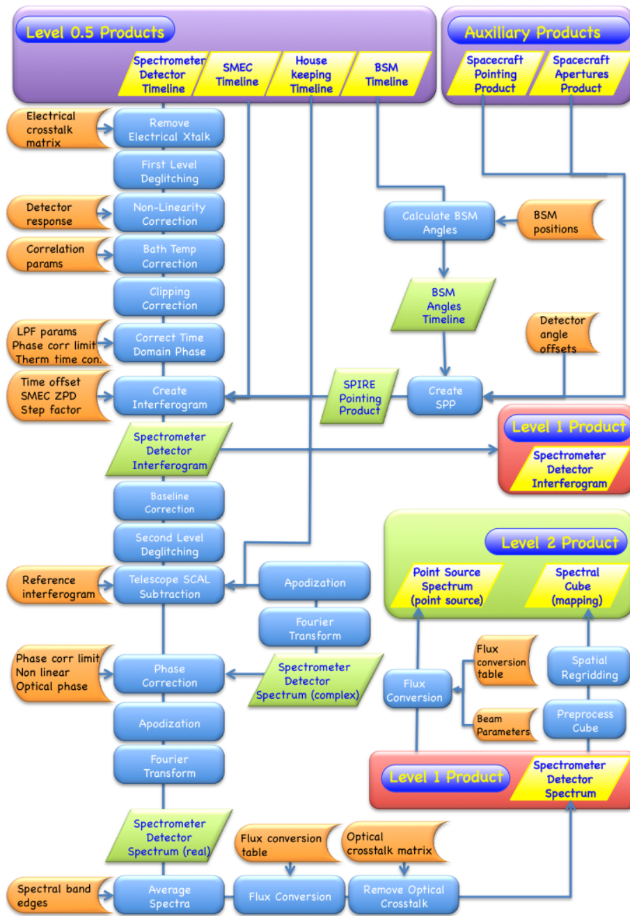
Figure 4.25. The SPIRE Spectrometer pipeline.
