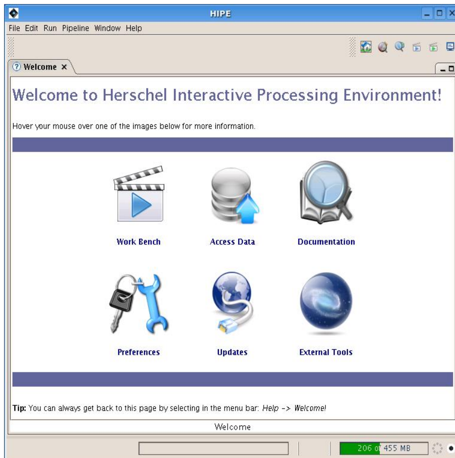
Figure 4. Information on 'Welcome' screen icons. See bottom strip of the HIPE screen for the explanation of each icon the mouse is placed over.
