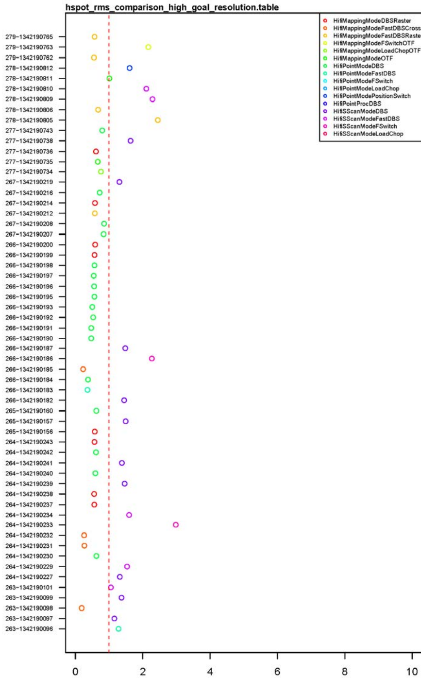
Figure 1: Ratios of measured to predicted (HSpot) noise for observations carried out in PV-II through February 25, with data smoothed to the goal low resolution (top) and high resolution (bottom). All testmode observations are included.
