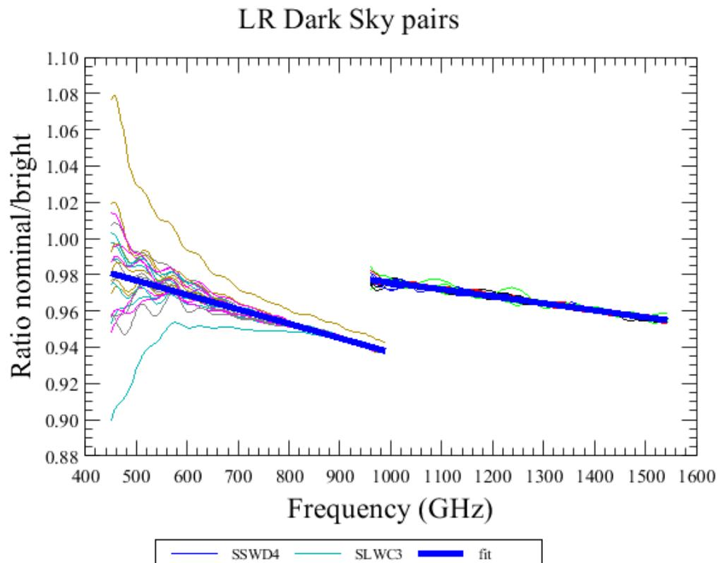
An empirical wavelength-dependent gain correction factor, to be applied after the Fourier Transform in the pipeline.
